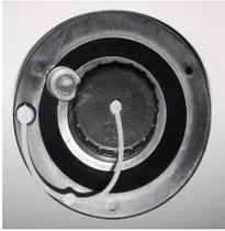
When traveling, you may want to drain the tank, or keep the quantity of water in it to a minimum. This reduces the total weight of the motorhome for travel. Make sure when draining the tank, that the water pump has been turned off. The fresh water tank drain valve is located below and near the fresh water fill spout. Water in the tank can be drained by turning the drain cock perpendicular to the motorhome body. To close the valve, turn the lever parallel to the motorhome body.
