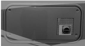
The furnaces used by Thor Motor Coach have electronic ignition, and there is no need to access this panel except for service. As with all appliances, service is best left for your dealer. To remove the panel to check for insect nests, you will need a Square or a Phillips head screwdriver. For further information, reference the furnace manufacturer's manual provided with your vehicle.
