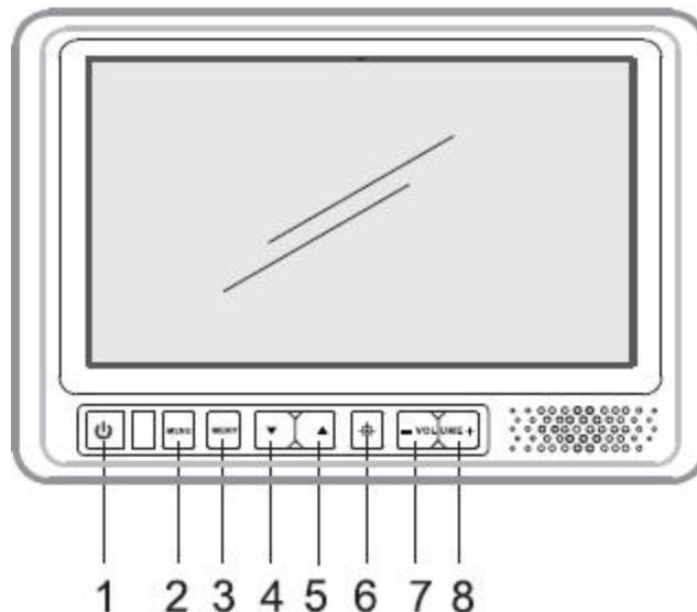
1. Power On/Off: Press once turns unit on.
