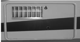
You can gain access to the water heater control panel to check for insect nests by turning the tab at the top and allowing the door to hinge down. Due to the electronic ignition, it is no longer necessary to access this compartment for lighting the pilot. It has an electronic module board, electronic ignition lighter, and a safety pop-off valve to relieve the pressure, should it be necessary.
