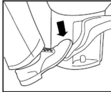
To flush the foot pedal style, depress the pedal all the way until rinse clears the bowl. Be sure to release the lever slowly. Movement of the flush lever opens the waste valve and allows the water to pass into the holding tank.
