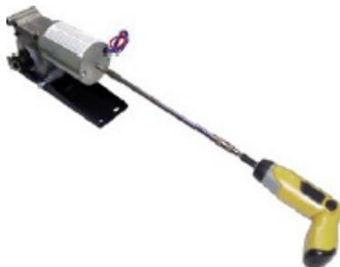
4. If the cables tighten, and the motor is difficult to turn, REVERSE THE DIRECTION. Over-torquing can happen, resulting in severe damage.
